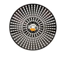
The AST Disc is used for AST and concentration determination.
