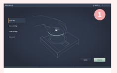
**Choose AST Disc and load** The AST Disc allows automated time-lapse imaging of bacterial population growth in wells containing different concentrations of antimicrobial agents.
