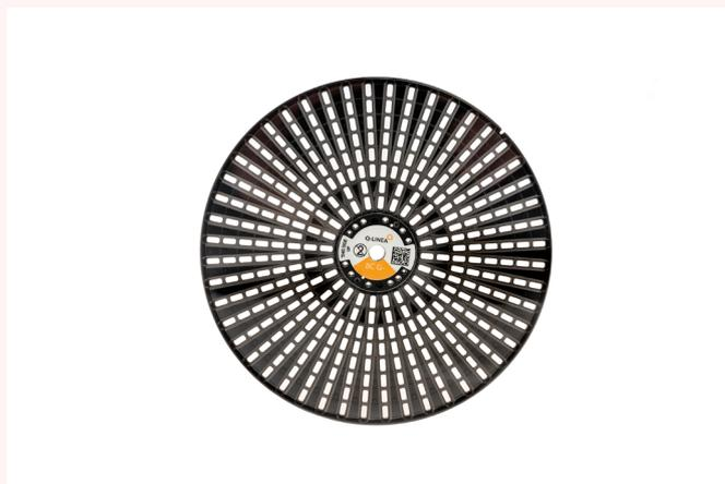
The AST Disc is used for AST and concentration determination.
