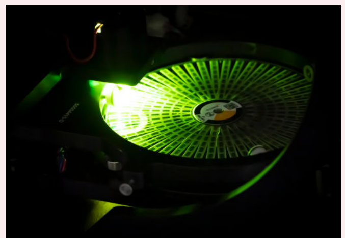
Figure 2. The Disc during AST reading. The unique proprietary technology allows automated time-lapse imaging of bacterial population growth in wells containing different concentrations of antimicrobial agents.
