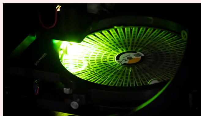
Figure 2. The Disc during AST reading. The unique proprietary technology allows automated time-lapse imaging of bacterial population growth in chambers containing different concentrations of antimicrobial agents.
