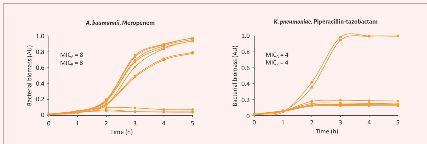
Biomass plotted over time for different specimen types and for a selected number of bacteria and antimicrobials combinations, each curve representing one concentration (mg/L). For each AST, ASTar-MIC (MIC<sub>A</sub>) and reference BMD MIC (MIC<sub>R</sub>) are noted.
